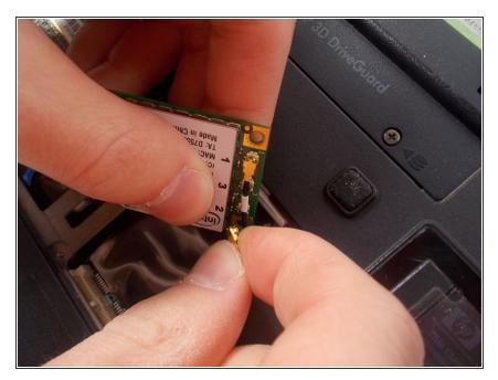
• Pull on each of the wires connected to the card. They will easily pop off and the WiFi card will be released.
