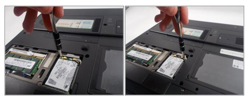
• Locate the screws at the top of the card and use your Philips screwdriver to remove them.
