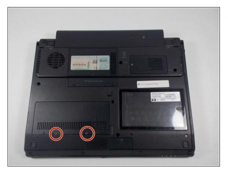
Flip the laptop over and locate the RAM cover plate towards the left of the laptop. There will be two screws located on the panel.
