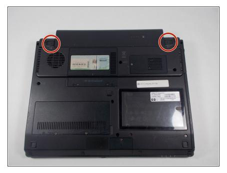
Flip the laptop over and locate the two battery release switches. It can be found to the left and right of the battery pack.
