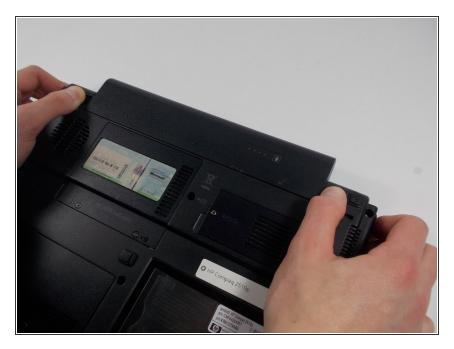
Slide each switch outward with your thumbs, the battery will now be loose and can be pulled out.
