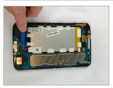
Unplug the battery connection carefully using the plastic opening tool.
