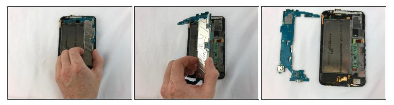
• Remove the motherboard from the device by carefully lifting it out.
