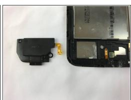
Remove the speaker using the plastic splunger
