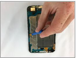
Before Changing the motherboard, you have to lift up the (ZIF) zero insertion force by using the
