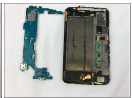
Remove the mother board from the device by carefully lifting it out.
