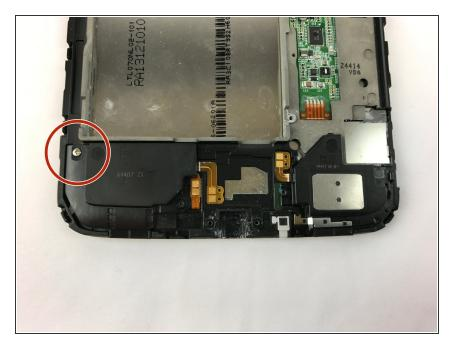
Remove the last screw holding down the speaker.
