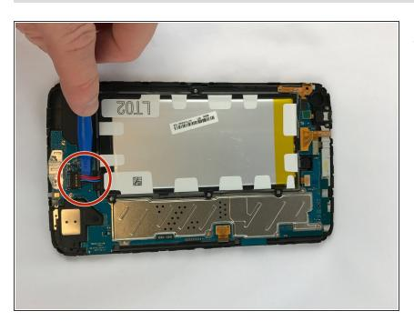
Unplug the battery connection carefully using the plastic opening tool.
