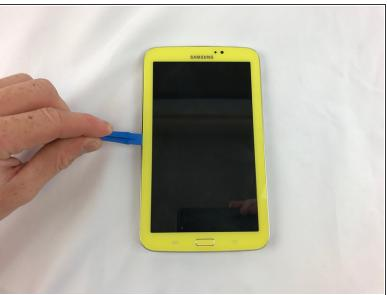
Using the plastic opening tool to open up the device, wedge in the seam between the screen and the back cover. Slide the tool around all the edges and remove the screen from the back cover
