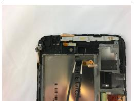
Remove camera by carefully lifting out of the device
