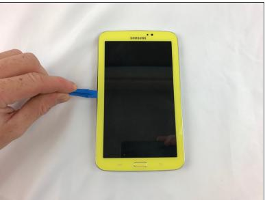
Using the plastic opening tool to open up the device, wedge in the seam between the screen and the back cover. Slide the tool around all the edges and remove the screen from the back cover
