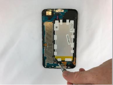
Unscrew the ten 4mm PH000 bolts holding the motherboard on the device
