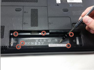
Unscrew the following 5mm screws with a #0 Phillips screwdriver.
