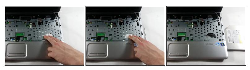
Slide the CD player case away from the device with medium-hard force, it should come right out.
