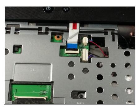
Similarly to how you remove the keyboard, gently pry a small section of the power button frame up.
