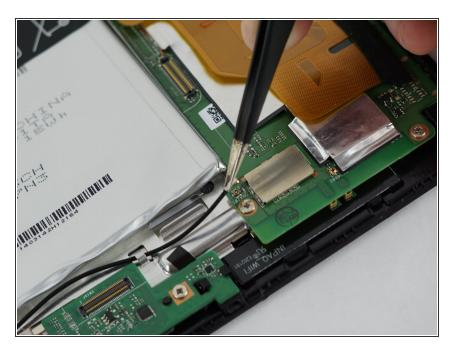
Using tweezers, detach the small black cable connected to the motherboard by gently tugging on it.
