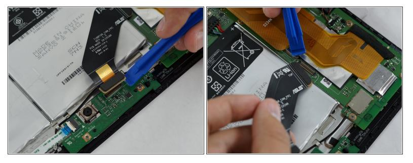
• To remove the right speaker, begin by detaching the large black strip connecting from the camera board to the motherboard using a plastic opening tool.
