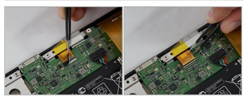
Disconnect the LCD connection apparatus by carefully removing the black protective strip with tweezers and gently tugging on the orange ribbon.
