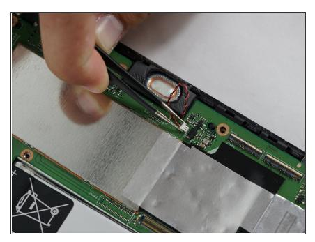
• Disconnect the speaker from the motherboard by gently tugging on the cable head with tweezers.
