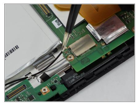
Using tweezers, detach the small black cable connected to the motherboard by gently tugging on it.
