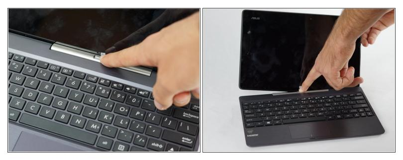
Detach and separate the screen from the keyboard by pressing the silver release button at the base of the tablet.
