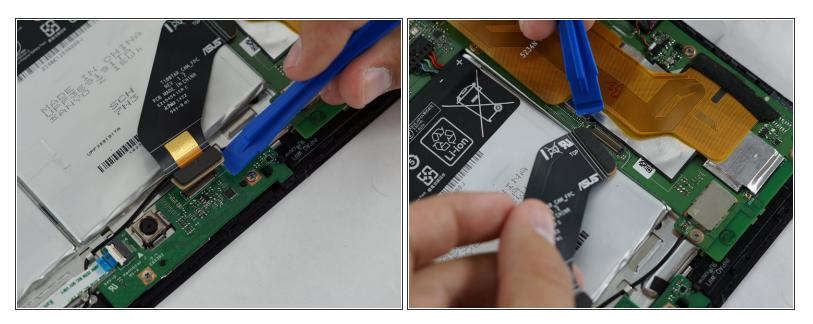
Using a plastic opening tool, carefully lift up and detach the large black strip connecting from the camera board to the motherboard.
