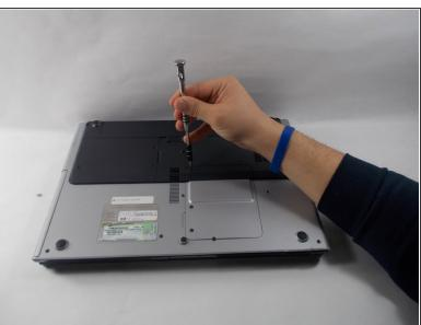
Unscrew the three 2x5mm screws with a #00 Phillips screwdriver.
