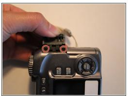
Remove the 3 mm long screws with a Phillips head screwdriver that has a PH000 size bit.
