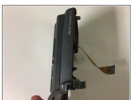
You have detached the back casing and LCD screen.
