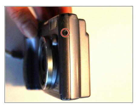
Remove the 3 mm long screw using Phillips head screwdriver that has a PH000 size bit.
