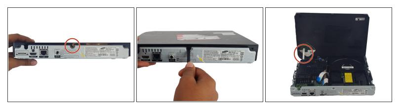
• Use the plastic spudger to pry open the top panel from the center tab.
