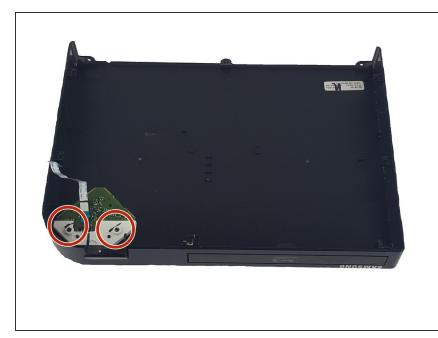
Use a Phillips Head #00 to unscrew the two 7mm screws on the media controls.
