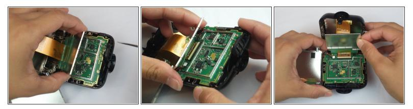
• Remove the metal case off of the motherboard.
