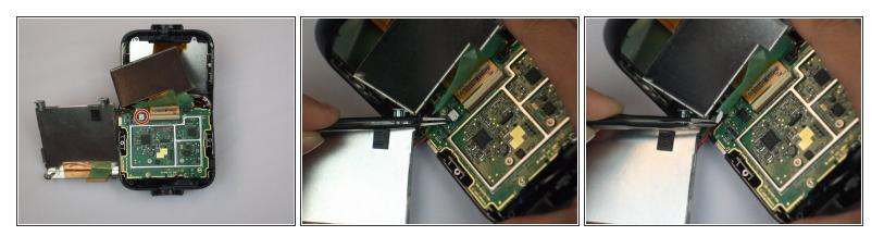
• Remove the battery connection.
