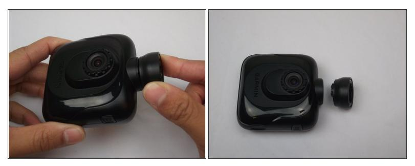
• Remove the Dash Cam socket piece.
