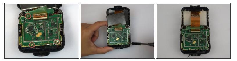
• Remove the three 5 mm screws using the Torx T5 screwdriver.
