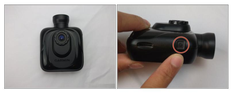
Be sure to turn off the Dash Cam by pressing the power button.
