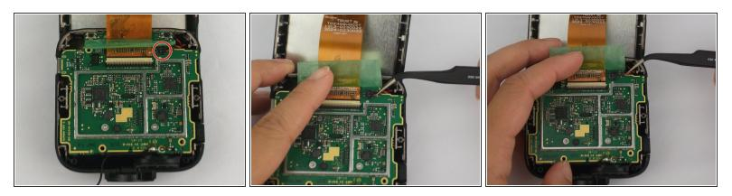
Use tweezers to remove the connector on the top right of the motherboard.
