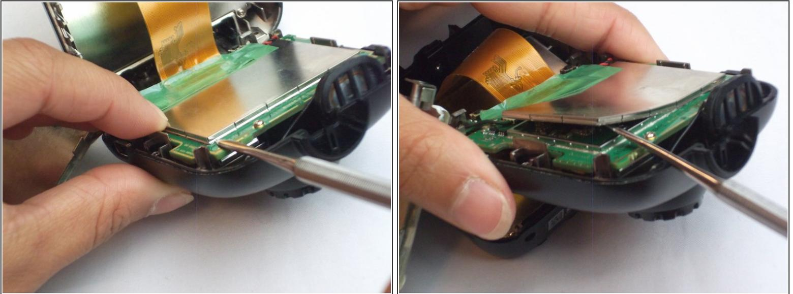
**⚠** This step shows the use of an incorrect tool. Always use an ESD safe tool, like a nylon spudger, when working with delicate internal components.
