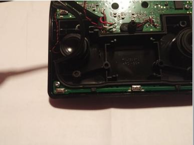
Carefully remove the rubber gasket using the tweezers.
