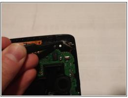
Remove the microphone from microphone slot using tweezers.
