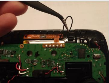
Use the tweezers to remove the antenna from the retaining clips.
