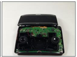
• Gently lift the front panel off of the device and carefully rest it to the side.
