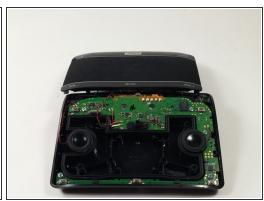
Gently lift the front panel off of the device and carefully rest it to the side.
