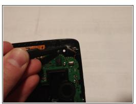
Remove the microphone from the microphone holding slot.
