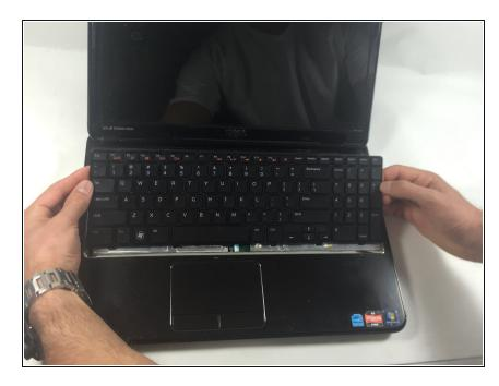
• Lift and slide the keyboard towards the screen to remove the tabs on the keyboard from the slots on the palmrest.
