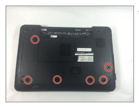
Turn the computer over and remove the six screws that secure the palmrest assembly
