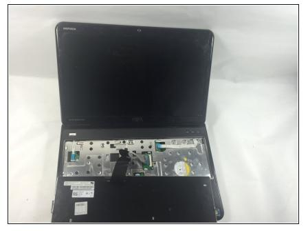
• Flip the keyboard over and place it on the front of the device making sure not to pull out the keyboard cable.
