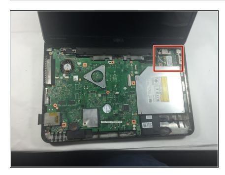
• Disconnect the display antenna cable from the Mini Card.
