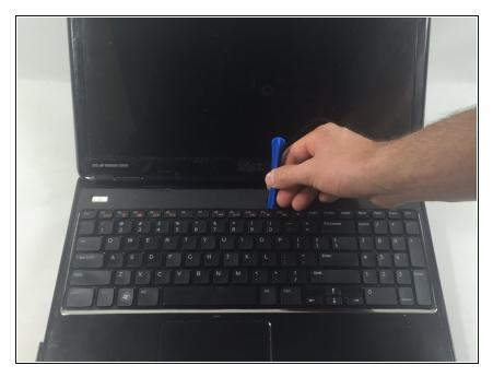
• Pry the keyboard away from the device using the plastic opening tool.
