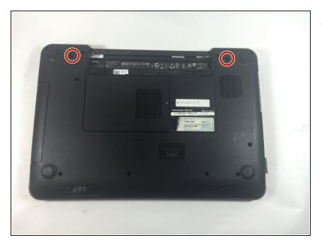
Turn the device over and then remove the two 5 mm Phillips #0 screws that keeps the display assembly to the base and then flip the device.
