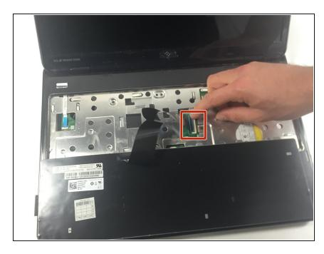
• Lift up the connector latch and remove the keyboard cable. The keyboard is now free from the device.
