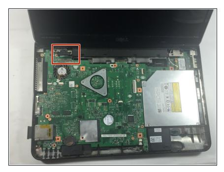
• Disconnect the LCD display cable and touch screen cable.
