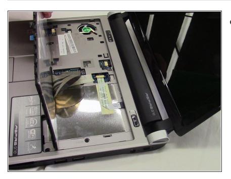
Gently remove the keyboard power ribbon that is attached to the motherboard.
