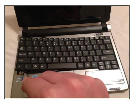
Lift the keyboard up with the spudger and lift along edges until the keyboard is free.
