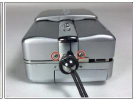
Unscrew the 7 4.1mm screws around the camera using a PH000 screwdriver.
