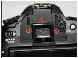
Identify and unscrew the ten PH000 screws around the top, front, left, and right sides of the camera body.
