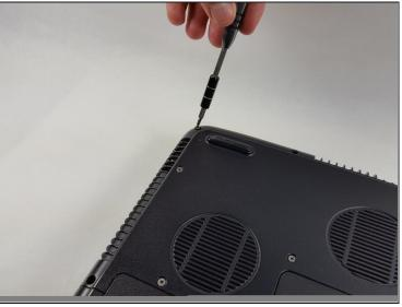
• Using a Phillips #0 screwdriver, unscrew all four Phillips PM 2.5X13.0mm screws and place in a secure area until the end of the project.
