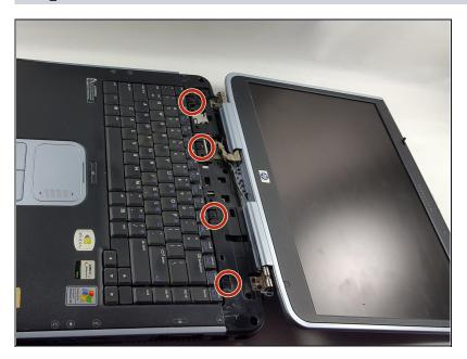
Use the Phillips #0 screwdriver again, unscrew all four Phillips PM 2.5X13.0mm screws from the top of the keyboard and set aside.
