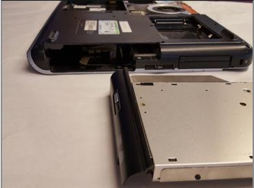
• Using your hands, firmly grasp the CD drive and pull outwards until it is completely removed.
