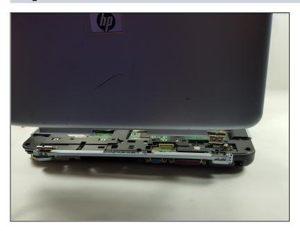
Firmly grasp the top of the screen with your hands and pull towards you and upwards to remove the screen from the base.
