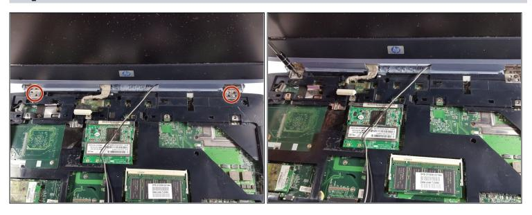
• Use the Phillips #0 screwdriver again to remove the four Phillips 2.5X13.0mm screws that hold the clips for the screen into place.
