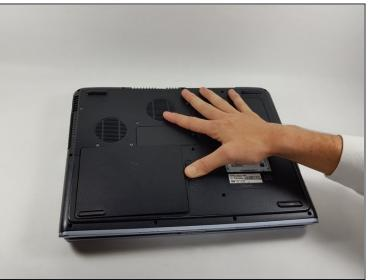
Press and slide up the battery release tab with your thumb until the battery pops out of place.
