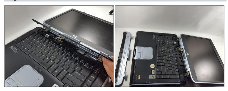
Use hands to completely lift off the strip cover and remove.
