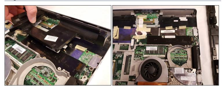
Grasp speaker assembly firmly and pull towards you and up to remove the speaker completely from the laptop.
