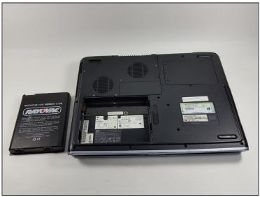
• Using two fingers, pry the rest of the battery out of the socket.
