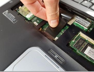
• Gently slide out the connecting cable from the laptop to the keyboard.
