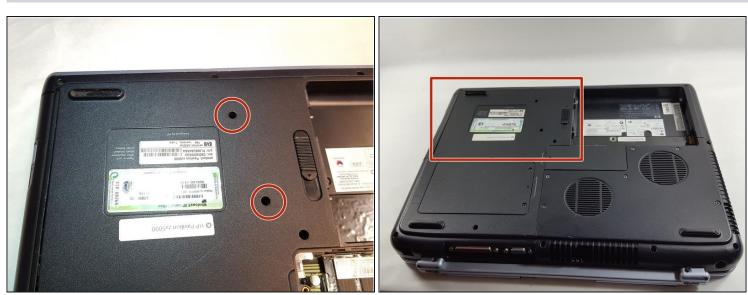
Unscrew the two Phillip PM 2.5X6.0mm screws in the top right that hold the optical cover in place using a Philips #0 screwdriver.
