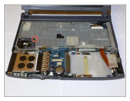
Remove this final screw and lift out the fan
