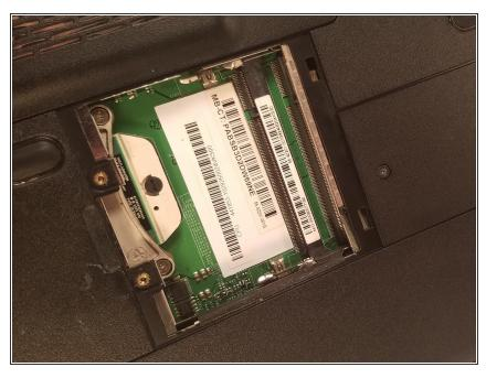
ithis is the device with both RAM sticks removed.
