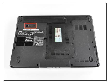
Locate the battery release switch on the bottom of the laptop.
