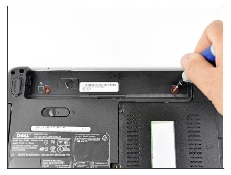
Remove the two 4.00 mm Phillips #1 screws from the battery tray.
