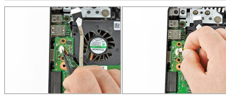
Disconnect the fan cable connector by pulling it towards the fan with a spudger.
