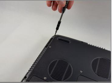
• Using a Phillips #0 screwdriver, unscrew all four Phillips PM 2.5X13.0mm screws and place in a secure area until the end of the project.
