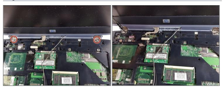
• Use the Phillips #0 screwdriver again to remove the four Phillips 2.5X13.0mm screws that hold the clips for the screen into place.
