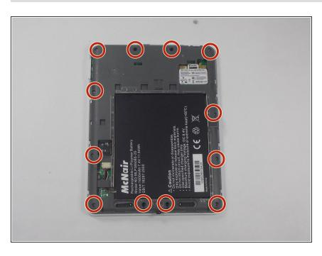
Using a Phillips #0 bit, remove the 12 4mm screws.
