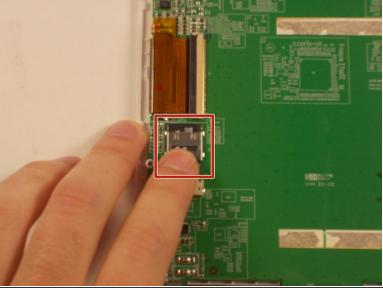
Push upwards on the SD card slot to release it.
