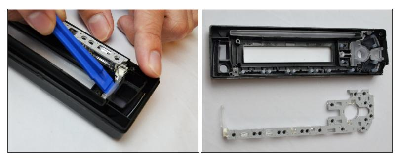
• Use the plastic opening tool to lift up and remove the cover.
