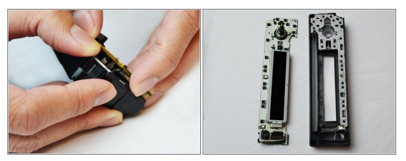
Lift and remove the motherboard to reveal the inside of the front panel.
