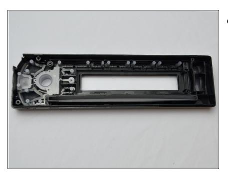
The buttons are now able to be removed and replaced if damaged or missing.
