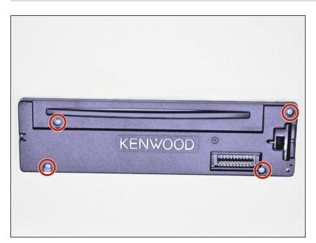
• Use the Phillips #0 Screwdriver to remove the four screws.
