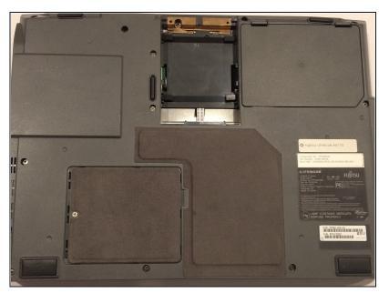
Close the screen of the laptop, then flip the computer over so that the bottom side is facing up.
