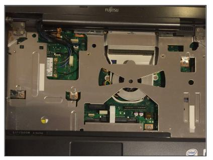
Flip the computer over again, like it was before removing the screws. The screen must be opened and pushed down so that it lies flat with the keyboard. Both the keyboard and screen must face up.
