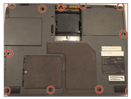
Using a Phillips #1 screwdriver, remove the eleven 1 cm screws located around the perimeter of the laptop's edge.
