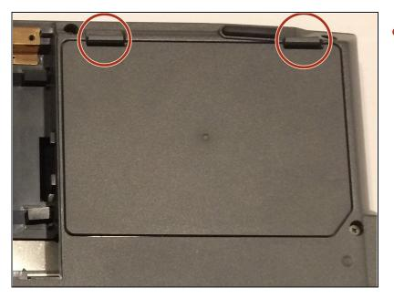
To remove the battery, place your fingers underneath the two clips and simultaneously lift them up while pulling the cover towards you.
