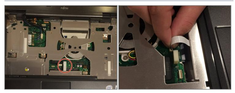
To remove the metal undercarriage of the keyboard, you must first detach the ribbon cable connected to the trackpad. Firmly grasp the base of the ribbon cable where it connects to the motherboard and gently pull it upward to disconnect it.
