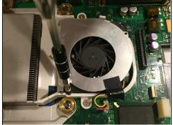
Located around the fan, there are two-three mm screws that need to be removed. Use a Phillips #1 screwdriver to turn these screws counter-clockwise and unscrew them.
