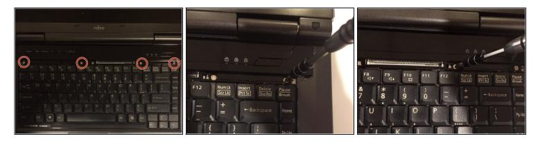
With a Phillips #1 screwdriver, unscrew the four-six mm screws that were hidden under the plastic piece you removed.
