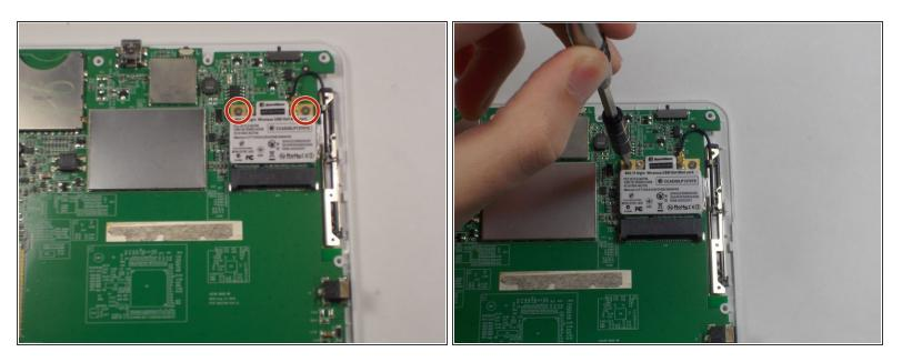
Using a Phillips #0 bit, remove the two 3mm screws at the top of the wireless card.
