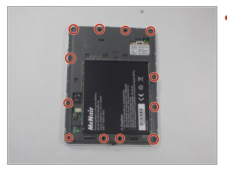
Using a Phillips #0 bit, remove the 12 4mm screws.
