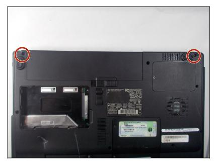
Remove the two 6mm screws that are directly under the screen.
