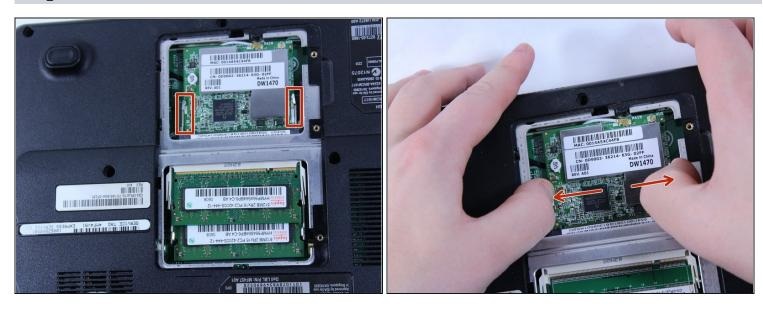
• To remove the wireless chip, push outward on its two metal brackets.
