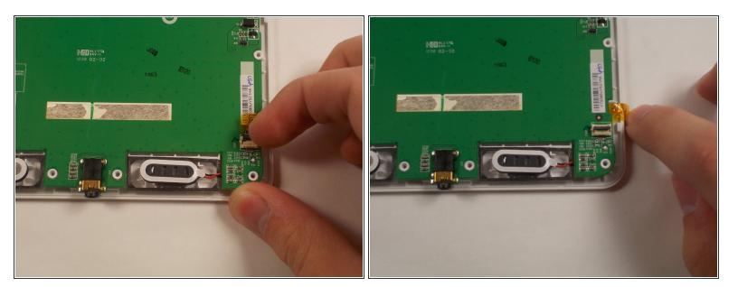
• Use the tip of your plastic spudger or your fingernail to flip up the shorter retaining flap. The smaller gold ribbon cable can now be pulled out safely.
