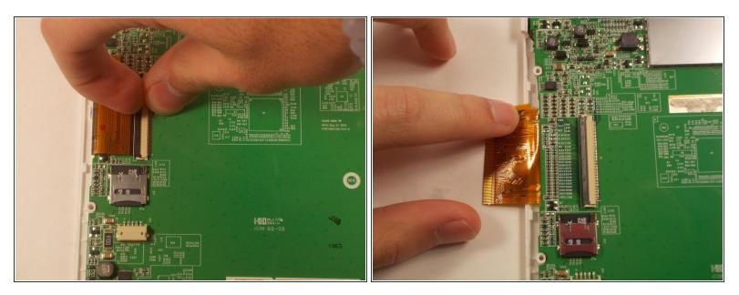
• Use the tip of your plastic spudger or your fingernail to flip up the long retaining flap. The longer, gold ribbon cable can now be pulled out safely.
