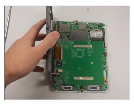
Now, lift up the gray piece, unplug the battery connector, so the gray piece will come free from the rest of the device.
