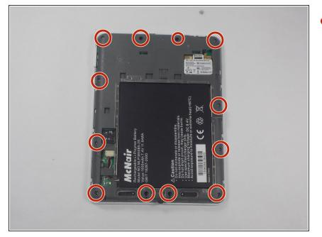
Using a Phillips #0 bit, remove the 12 4mm screws on the outer area of the gray area exposed by removing the back panels.
