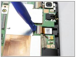
Use a plastic opening tool to lift the black retaining flap on the ZIF Connector
