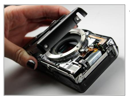
Using your hand, gently lift up the front cover and separate it from the camera.
