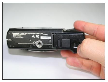
On the bottom of the camera, use your finger to push the lock button to the open position which will cause the hinged door to swing open.
