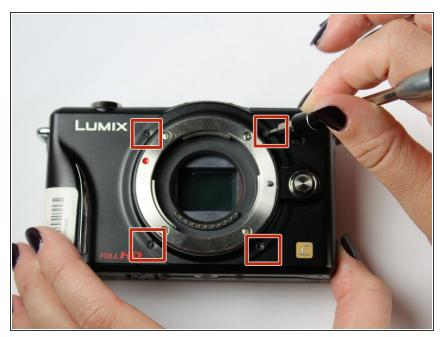
Using a Phillips #00 screwdriver, remove four black 2.69 mm screws from the front of the camera.
