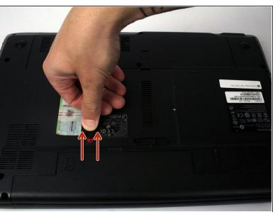
Slide the battery unlock latch to expose red, as shown.
