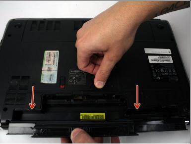
Slide battery release to open, then remove the battery.
