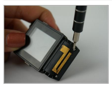
Use a PH000 screw head to undo the newly revealed silver 4 mm
