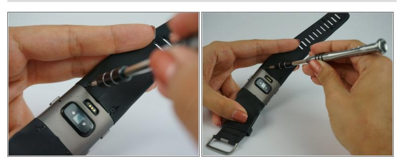
Unscrew all four black 3 mm Phillips screws on the underside of the watch using a T5 screwdriver.
