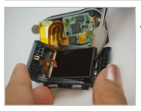
Remove the LCD screen from the clock face.
