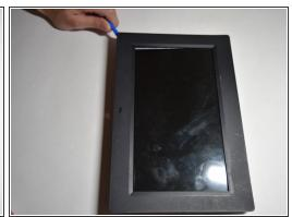
Using the black nylon spudger, pry off the clips all around the frame. You will hear a popping sound for every clip
