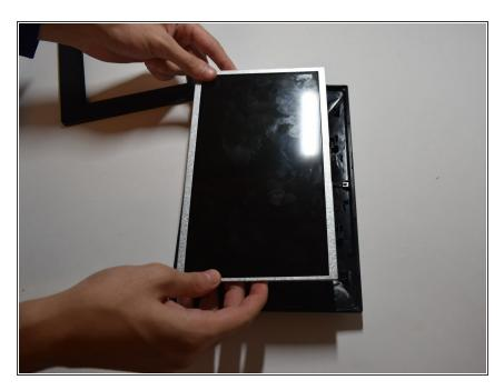
Lift screen out of place so you can access the plugs that connect it.
