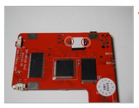
On the back end of the mother board unsolder the USB port at the two points shown.
