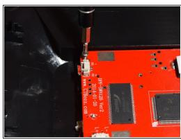
Using the ph0 phillips head screwdriver unscrew the four 4mm screws circled in the picture.
