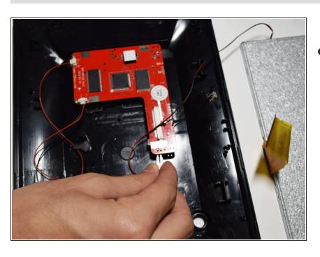
Disconnect the red and black cable connecting the screen to the motherboard by just pulling it out.
