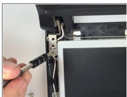
Unscrew each of the four 6.5mm Phillips #0 screws securing the screen to the case.
