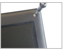
Take out the four 4.5mm Phillips #0 screws located at the corners of the screen.
