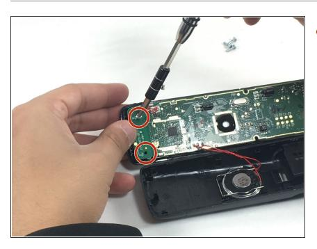
Unscrew a second set of 10mm screws to access to the other side.
