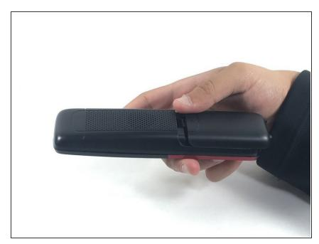
• Slide the back cover off the cause.
