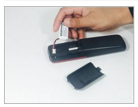
lift the battery and unplug the two pin cable from phone base.
