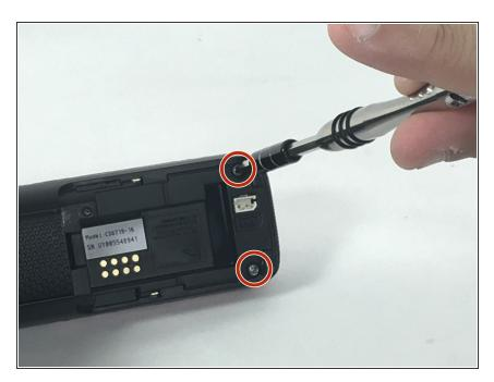
Remove the two 10mm screws at the base of the phone.
