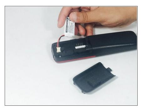
Now remove the battery by lifting it and removing the two pin cable.
