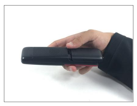
Remove the sliding cover on the back of the phone case.
