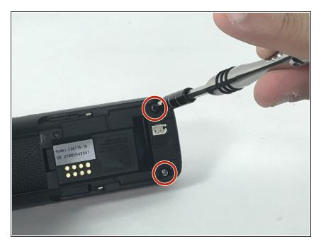
Unscrew the two 10mm screws on the back of the phone base.
