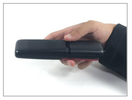
• Remove the back case of the phone to expose the battery.
