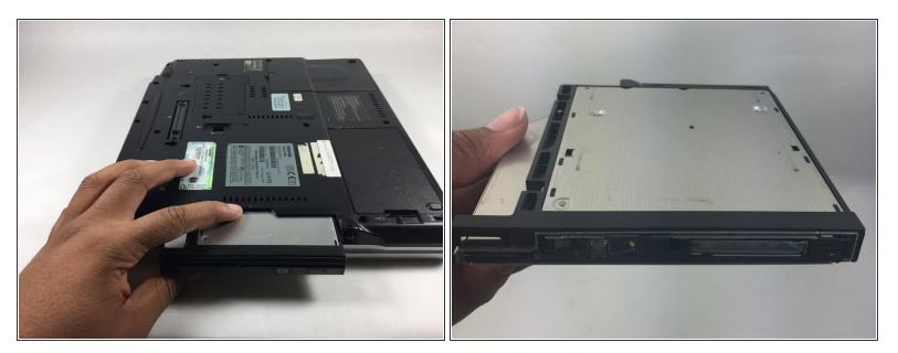
• Use your hand to remove the disk drive by pulling outward.
