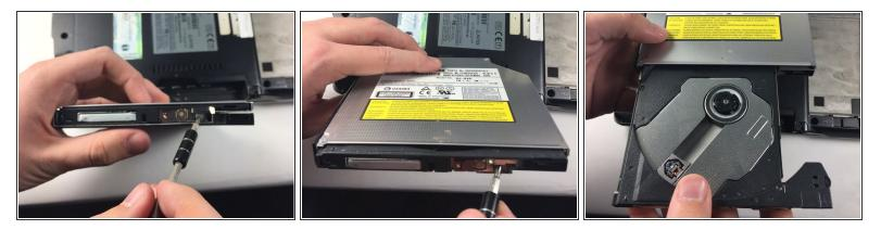
• Push the end of a paperclip into the small hole on the disk drive to open it if there is a disk that is stuck in the drive.
