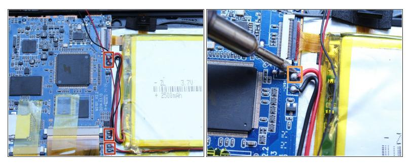
Using a soldering iron, desolder the contact points of the speaker, battery and screen on the motherboard
