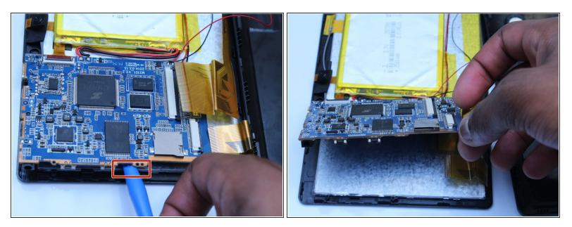
• Using the flat side of the spudger, lift up the mother board to disconnect from the screen.
