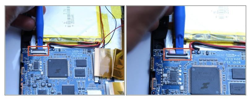
• Using the spudger, disconnect the ribbon cable connecting the camera to the motherboard
