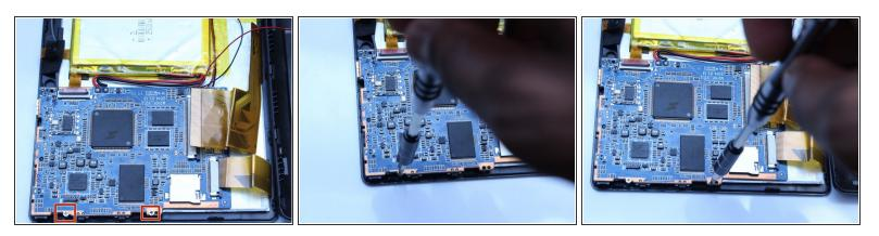
Use a Phillips screwdriver (PH00) to unscrew the two screws that connects the motherboard to the device
