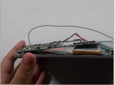
• Use plastic spudger to take off motherboard by lifting off right hand side and pulling sideways.
