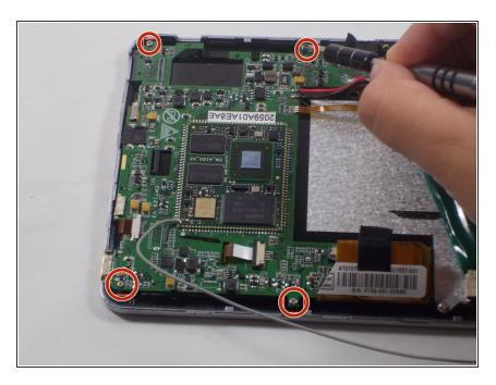
Unscrew 4 screws connecting around mother board using the J0 Phillips head screwdriver.
