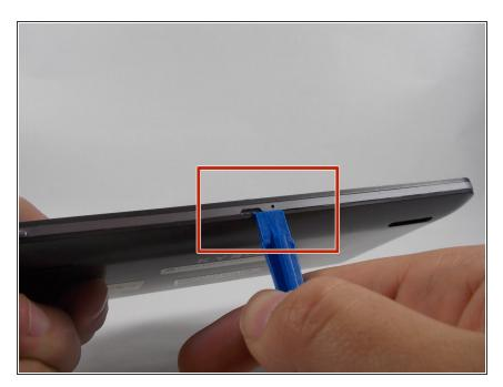
Use iFixit plastic opening tool to make small opening in the side of the device, and continue opening back panel
