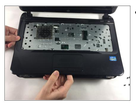
• Lift upwards to remove the palm rest.
