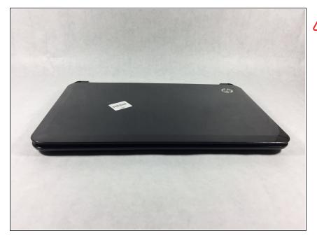
Power down the laptop and detach the charging cord (failure to do so can result in electrical shock).
