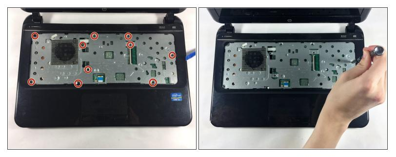
• Unscrew the 10 6.0 mm screws under the keyboard housing with a Philips #0 head screwdriver.
