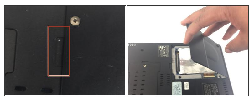
Locate the indent where the hard drive can be removed. Remove the cover.
