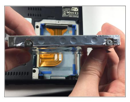
Locate the screws on each side of the encasing of the hard drive.
