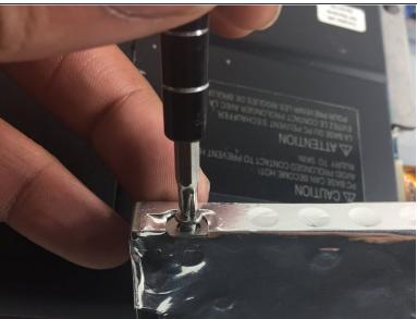
Use your Phillips screwdriver to remove the screws and be careful not to lose the screws.
