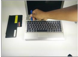
Use a plastic opening tool tool to pry around the edge of the keyboard.
