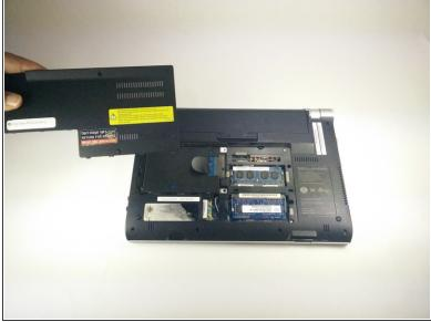
Use a plastic opening tool to pry up on the plate and remove from device.
