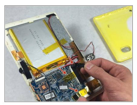
Remove the pieces of tape attached to the motherboard so that it can be taken off.
