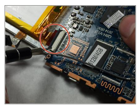
For the third connection, to the battery, the plastic piece that holds the wire strip in has a blue tab that rotates upward to release. The pivot point on one side is shown using the screw driver.
