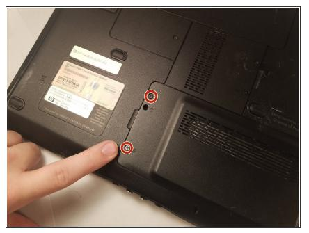
• Remove the two Phillips screws located on the back of the laptop.
