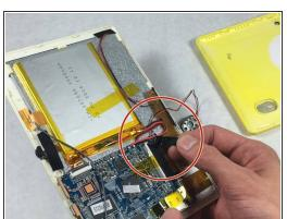
Identify the pieces of tape holding the battery to the back of the screen, and peel them off to remove them.
