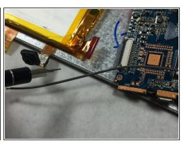
Locate the connection between the battery and motherboard, and disconnect it by pulling the two apart.
