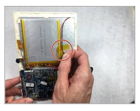
Once the back casing has been removed, identify the location of the battery inside the device, marked with the red circle.
